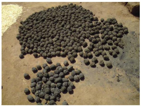
Charcoal dust and fines are saved by mixing with clay and forming into balls which are then allowed to dry. These are also sold.
